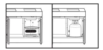
If gas cylinder not used, the hole can be covered with ABS cover supplied.
