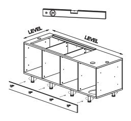
Ensure the height from the ground to the top of the carcass is minimum 735mm high in order to ensure at least 5mm gap from the bottom of the waterfall to the ground
